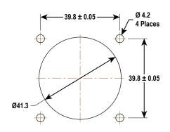
UPT07D-24-48P Size 24, 48 Way, Jam Nut Receptacle
